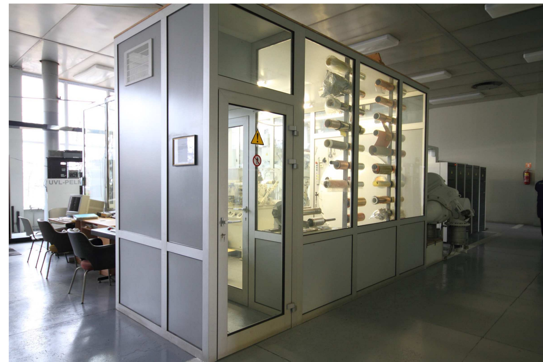
Fig. 2. Dry room in Sidrabe facilities.
