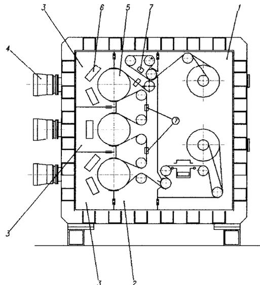
Figure 2: Layout of 3-drum's web coater: unwinding/rewinding compartment (1); intermediate compartment (2); deposition compartment (3); vacuum pumps (4); process drums (5); magnetron sputtering devices (6); optical and electric sensors for coating layers (7).
