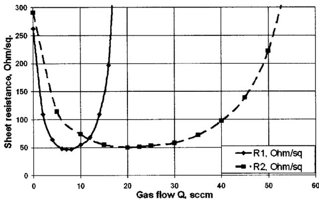
Figure 1: Dependence of ITO layer sheet resistance on oxygen flow (R1) and carbon dioxide flow (R2) into a vacuum chamber.
