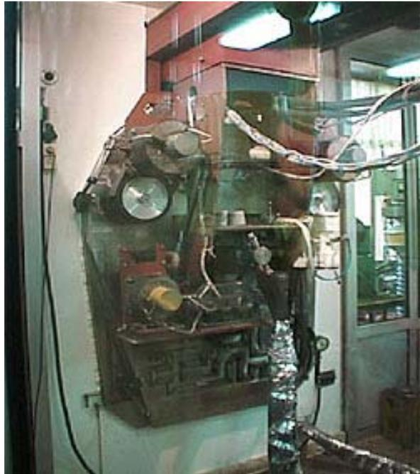
Figure 4 Vacuum pilot lithium deposition machine.
