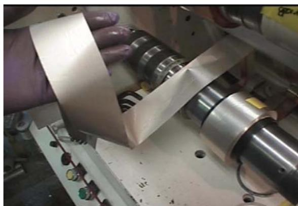
Figure 10 Double side coated Li on Cu foil.
