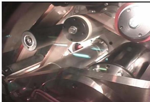
Figure 9 View through port of web in Li coater
