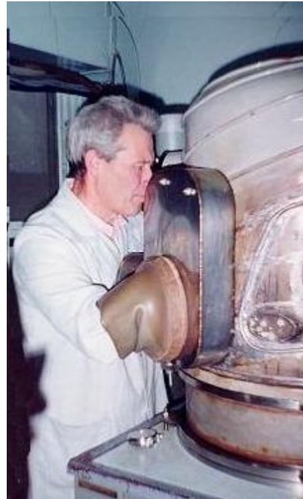
Figure 2 Bell Jar for Lithium evaporation
