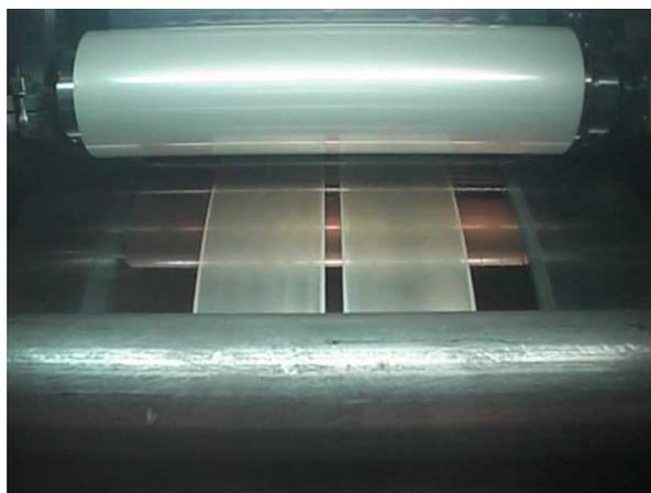
Figure 7 Lithium coated film during winding
