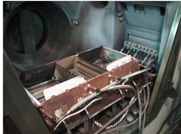
Figure 6 Lithium evaporation device.
