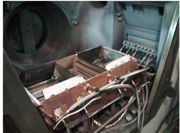
Figure 6 Lithium evaporation device.
